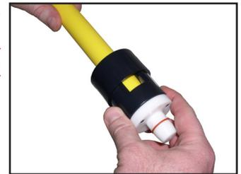
**4b** Chamfer end of pipe using [Continental's double ended ID chamfering tool.](#)
