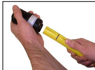
**6** If using ID chamfer tool with gauge, check for proper chamfer by inserting pipe on gauge up to the o ring. With proper chamfer, o ring will begin to enter pipe.
